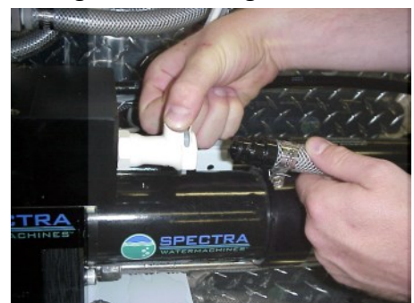
Connecting brine discharge service hose:
